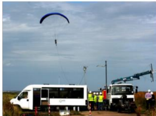
Figure 4: Crosswind device with ground-based generation. Image: KPS
