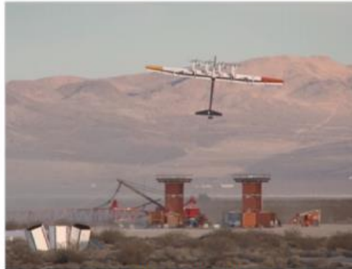
Figure 3: Crosswind device with on-board generation. Image: Makani
